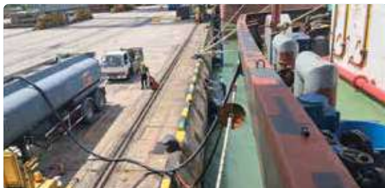
Sludge oil transfer to shore facility
