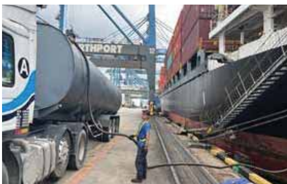
Sludge oil transfer to shore facility
